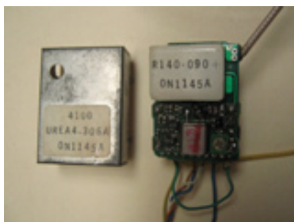
Complete Local Oscillator Module in 900 MHz marked as UREA4-306A, extracted from an old cell phone.
